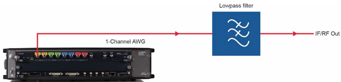
Figure 10. AWGs can generate radar (and any RF) signals following two different basic schemes
