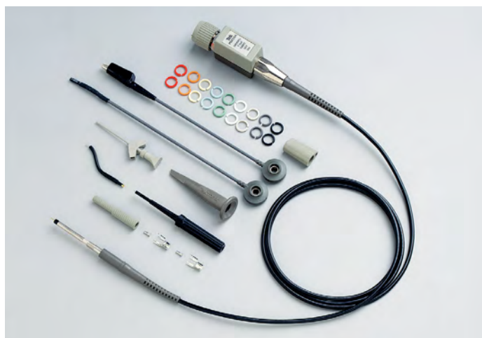
Figure 40. A typical passive probe with accessories.
