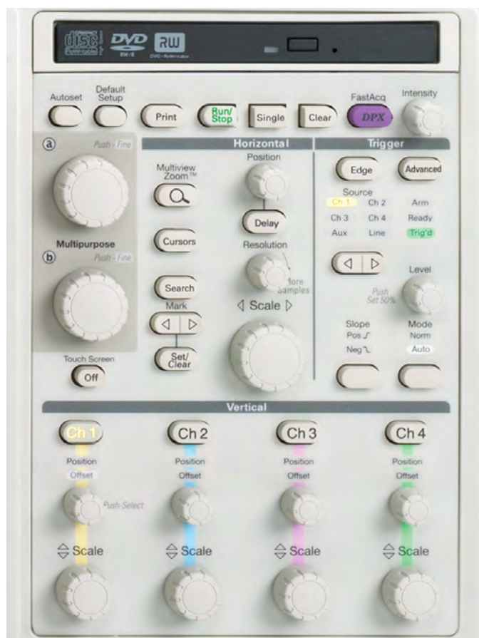
Figure 20. Front-panel control section of an oscilloscope.
